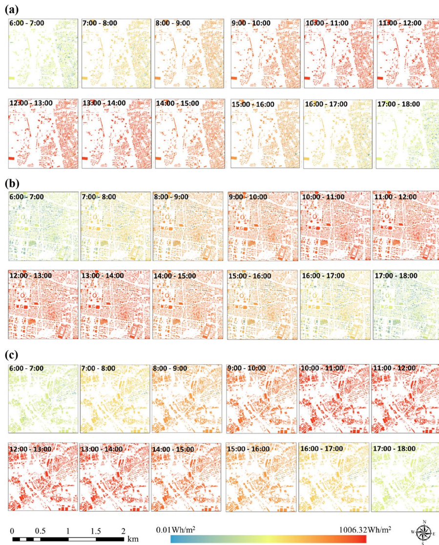
Fig. 6 Hourly solar irradiation distribution from 6 am to 6 pm. a Industrial area. b Commercial area. c Residential area
