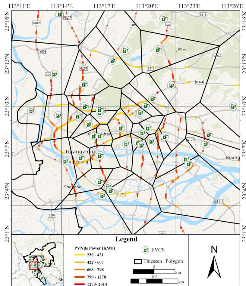
Fig. 6. Photovoltaic noise barriers (PVNBs) and electric vehicle charging stations (EVCSs) matching results for the PVNBs power maximization consumption scenario.
