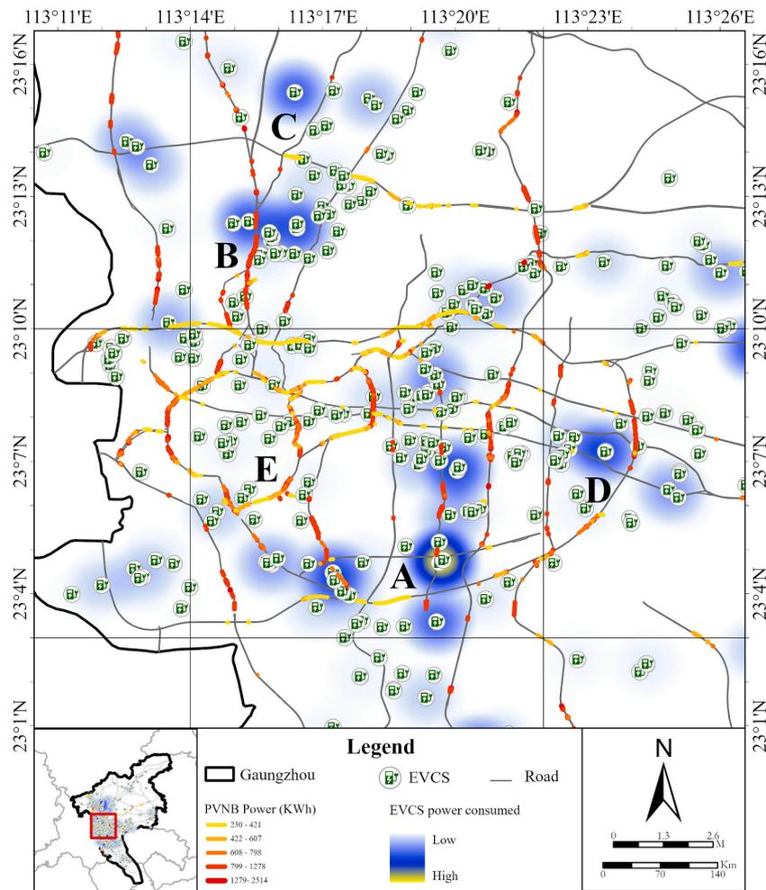
Fig. 5. Spatial distribution characteristics of electric vehicle charging stations (EVCSs) and photovoltaic noise barriers (PVNBs) in Guangzhou.
