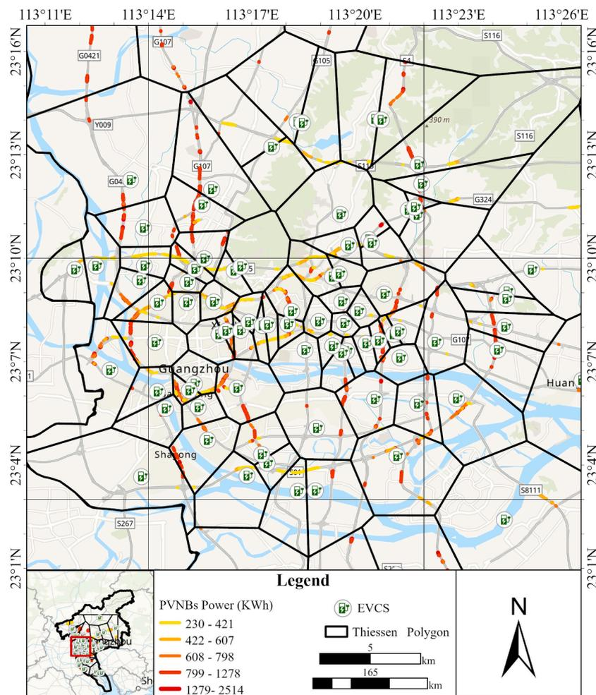
Fig. 7. Photovoltaic noise barriers (PVNBs) and electric vehicle charging stations (EVCSs) matching results under PVNBs-energy storage-charging station (PVNBs-ES-CS) future utilization scenario.
