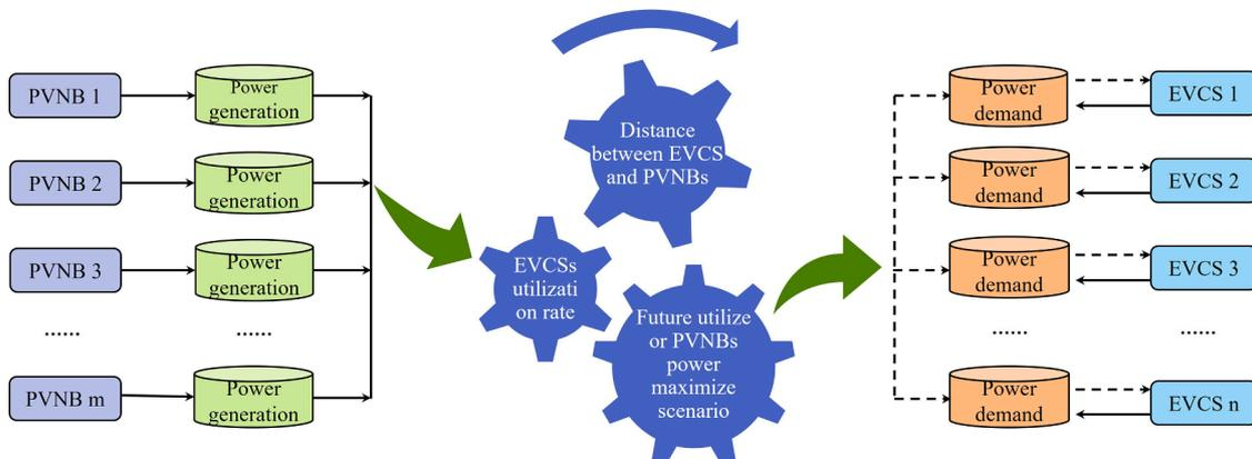
Fig. 3. Diagram of the photovoltaic noise barriers (PVNBs) and electric vehicle charging stations (EVCSs) matching process.
