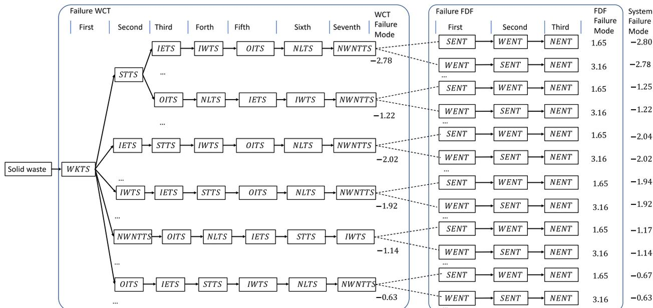
**Fig. 7.** Selected results of event-tree analysis (top 12 failure modes with the smallest reliability index) in 2014 based on optimized demand distribution results.
