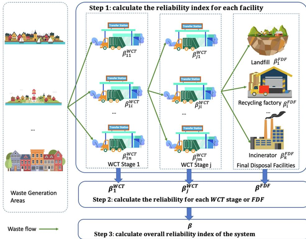
Fig. 1. Schematic diagram showing the reliability of a solid waste collection system ( $\beta$ : the reliability of the overall solid waste management system;  $\beta_j^{WCT}$ : the reliability of waste collection and transportation (WCT) stage  $j$ ;  $\beta^{FDF}$ : the reliability of final disposal facilities (FDFs)).
