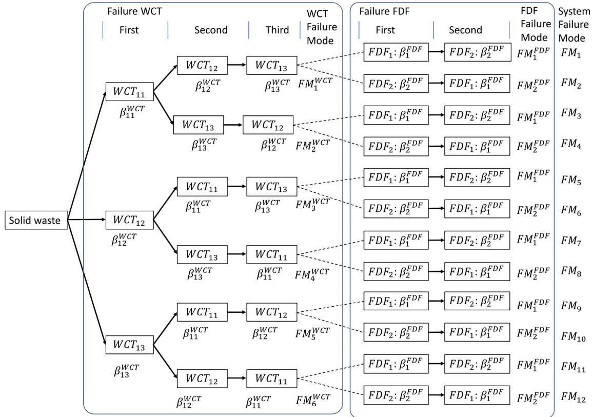
Fig. 3. An example of the failure event-tree for a waste management system with three transfer stations and two final disposal facilities.
