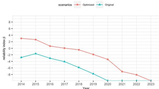
**Fig. 5.** Comparison between the optimized results and the original reliability index.
