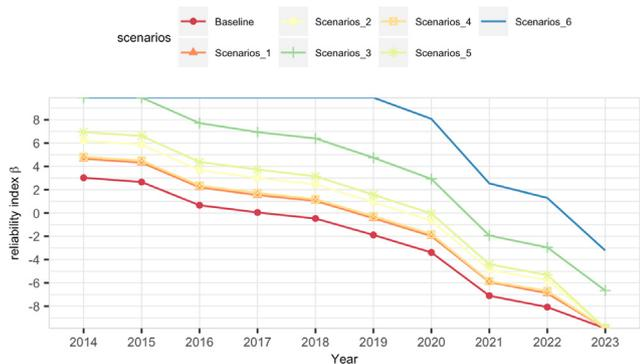
**Fig. 6.** Analysis of the impacts of facility capacity and recycling rate on the reliability index (Scenario\_1: increase capacity by 10%, Scenario\_2: increase capacity by 20%, Scenario\_3: increase capacity by 50%, Scenario\_4: decrease demand by 10%, Scenario\_5: decrease demand by 20%, Scenario\_6: decrease demand by 50%).
