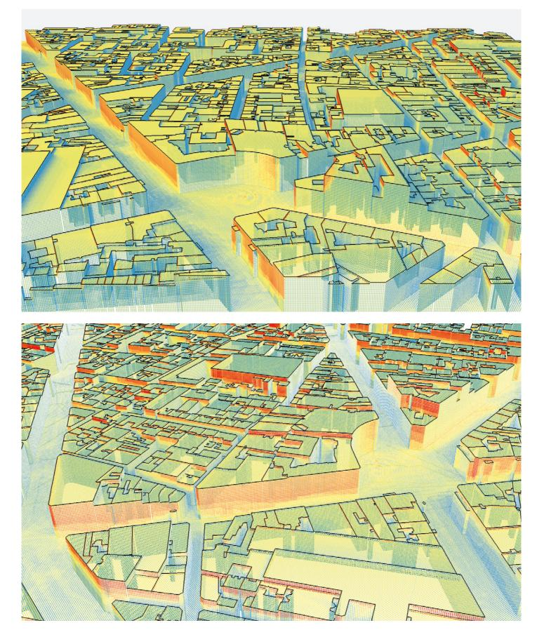
3D visualizations of annual solar irradiation in Paris, created as part of a study by MIT Senseable City Laboratory. They show specific instances of irradiation from two different perspectives.
