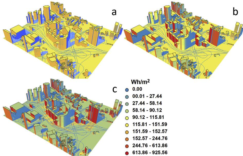
**Fig. 4.** Visualization of the point clouds in three modelling processes. (a) Point clouds in the shadow are in blue, and point clouds in the sunshine are in yellow. (b) Distribution of solar irradiation from the atmosphere. (c) Distribution of solar irradiation after four iterative reflections. (For interpretation of the references to colour in this figure legend, the reader is referred to the Web version of this article.)
