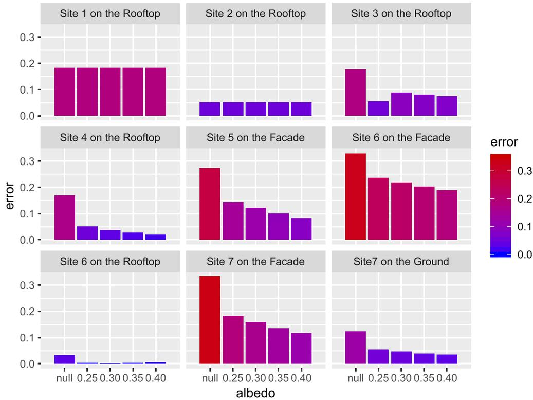
Fig. 7. Relative errors between the observed and estimated solar irradiancies. The bars marked with *null* in the x-axis were derived from ArcGIS software without the functionality of multiple reflections; the remaining bars represent the estimations that account for reflections with different albedo values, ranging from 0.25 to 0.40.
