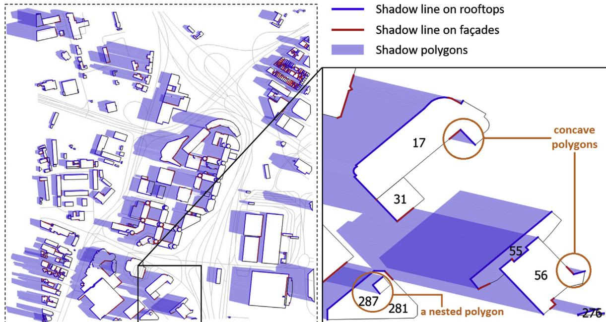
**Fig. 3.** Shadows of buildings visualized in 2D. Each shadow is represented by a 3D polygon, where space below the polygon is in the shadow. Blue lines and red lines are intersection lines where 3D polygons intersect with the buildings on the façades and rooftops, respectively. Concave and nested polygons are also marked with the orange circles. (For interpretation of the references to colour in this figure legend, the reader is referred to the Web version of this article.)
