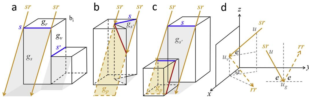
**Fig. 2.** The method used in the multiple reflection model. (a) A 3D shadow polygon  $g_s$  made by a convex rooftop. (b) A 3D shadow polygon  $g_s$  made by a concave rooftop. (c) A 3D shadow polygon  $g_s$  interrupted by the other building. (d) Reflective radiations on the façade and ground.
