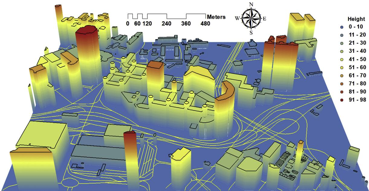
Fig. 6. 3D point clouds of the field test sites. The area (945 m × 775 m) contains 302 buildings with heights ranging between 2 and 94 m. Both horizontal and vertical resolutions of the 3D point clouds are 1 m, which thus generates more than 1.4 million point clouds in total.
