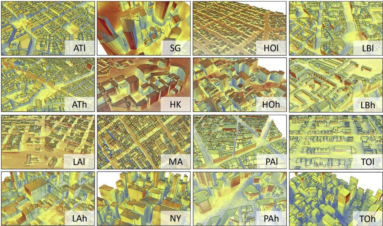
Fig. 5. Annual irradiation, as resulting after the process of multiple reflections, in the 16 study areas of ten cities is visualized, with a detailed spatial scale of 500m × 500 m.
