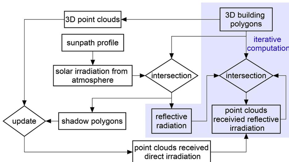
Fig. 1. Flowchart of constructing a 3D solar city presented by point clouds.
